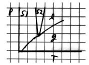
Not plausible. At most three phases of a single, pure compound can co-exist at equilibrium. This phase diagram has a quadruple point, i.e., a point at which 4 phases are in equilibrium. This would predict -1 for the number of 'degrees of freedom' from the Gibbs' phase rule, which is impossible:
